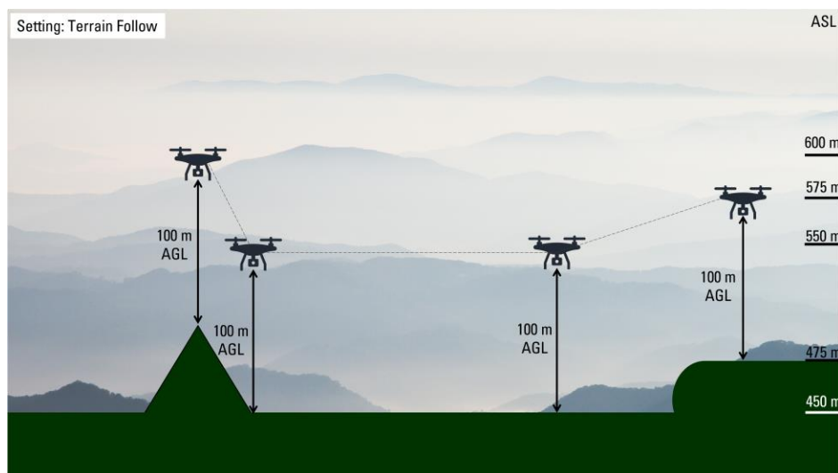
Figure 4 Example of drone altitude when using terrain follow setting.
